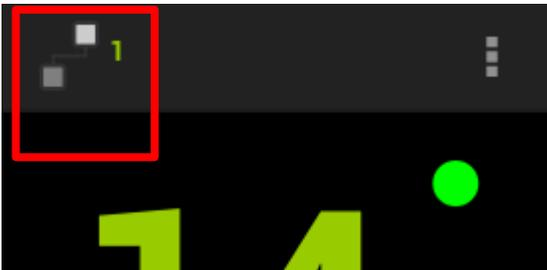
The TCP connection indicator shows the number of concurrent connections the scale has in process. You can have multiple computers connect to the scale at the same time. Each connection will increment this number indicated on the indicator. When the connection drops, **the number may not immediately update**. It may take some time to drop this number to the actual number of connections the scale is actually maintaining.
