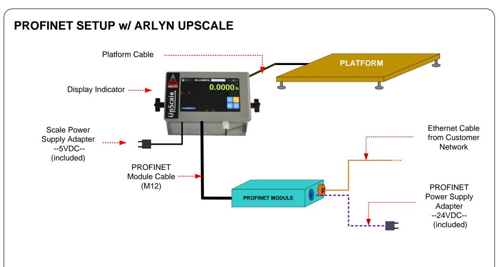
Platform Cable – Connects the PLATFORM to the INDICATOR through an M12 Cable.
