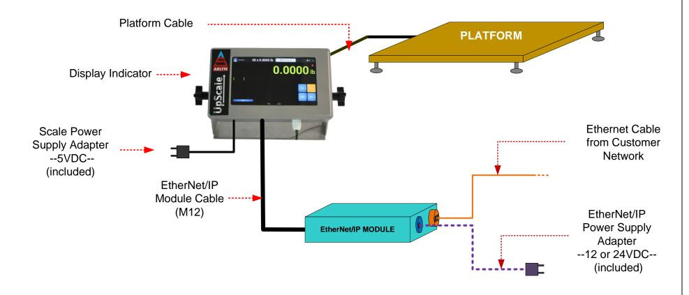
Platform Cable - Connects the PLATFORM to the INDICATOR through an M12 Cable.
