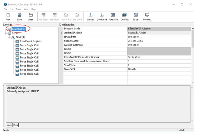
3) In the **Assign IP Mode** (on the right panel, 2<sup>nd</sup> row), select the dropdown to "Manually Assign". Then set your Static IP information as desired.
