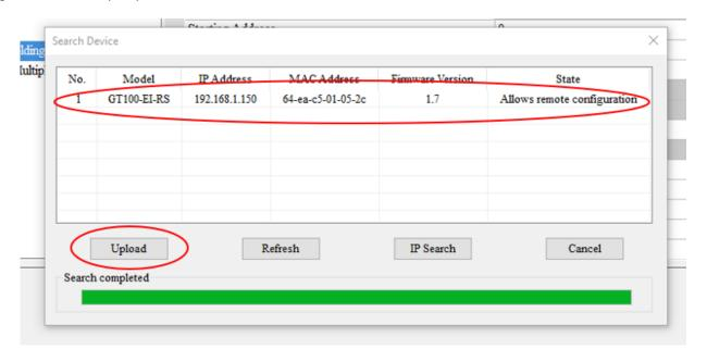
b. Select your EtherNet/IP adapter. NOTE: If you do not see the adapter here, it means the EtherNet/IP module has a different subnet IP address compared to your PC. Please call 1-800-645-4301 for further Technical Support
