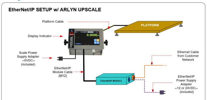
Platform Cable - Connects the PLATFORM to the INDICATOR through an M12 Cable.
