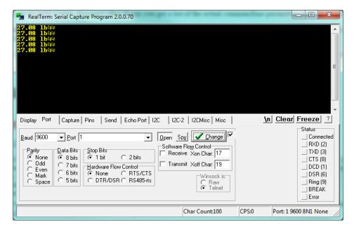
Make sure the **Port** designation on the bottom right of the screen shows the correct connection parameters. Then press the PRINT button on the scale to start sending data on to the terminal.
