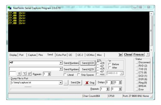
Press the **Send ASCII** button to send the command to the scale. If everything works out as specified, the scale is working properly.
