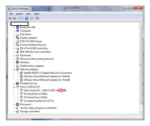
Note down the COM number of the device marked "Arlyn Scale V12 – USB (COMx)". The "x" denotes the number your PC has assigned to the scale. For the Arlyn UpScale Indicator, this will only show PCI Serial Port (COMx).
