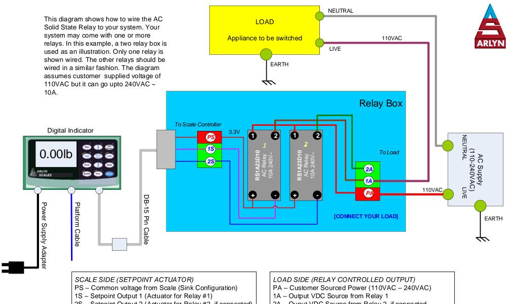
2S - Setpoint Output 2 (Actuator for Relay #2, if connected)
