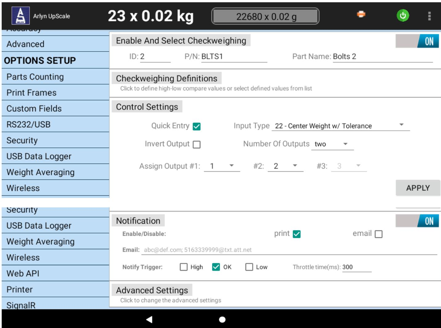
There are 5 sections to the Checkweighing Settings screen.
