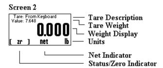
WEIGHT DISPLAY Shows the weight on the platform in the current units setting.
