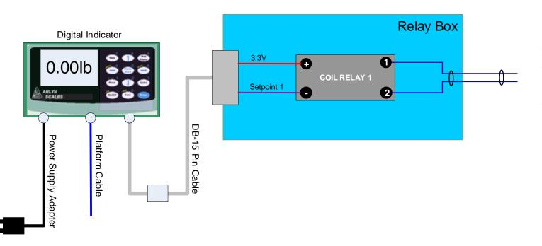
When Setpoint is activated from the scale, the Coil relay will actuate causing these two terminals (1 and 2) to short.
